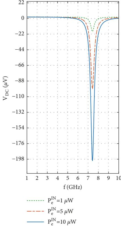
FIGURE 4: Frequency dependence of the amplitude of rectified signal  $V_{DC}$  generated across the MTJ caused by microwave heating of the spin-torque diode at different values of the input microwave power  $P_e^{IN}$  and the magnetic field  $B = 50mT$ , where the parameters of MTJ were taken from [14, 21] and the temperature  $T_0$  is equal to 300 K.
