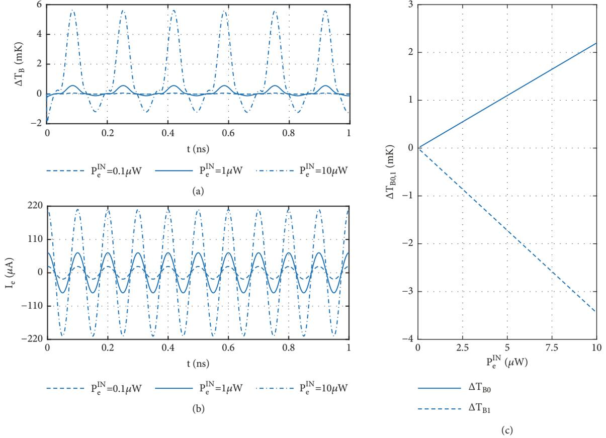
FIGURE 2: (a) Time evolution of (a) the temperature drop  $\Delta T_B = \Delta T_{B0} + \Delta T_B(\omega)$  across the tunnel barrier of MTJ and (b) an alternating current with a frequency of 6 GHz at a variable power. (c) Dependence of the magnitude of the constant and variable first-harmonic temperature drops  $\Delta T_{B0}$  and  $\Delta T_{B1}$  on the heating power.
