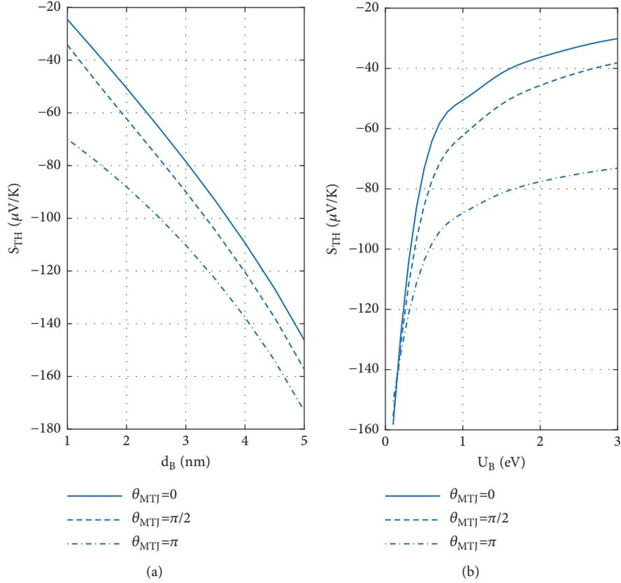
FIGURE 3: Dependence of the frequency-independent Seebeck coefficient  $S_{TH}$  on (a) the thickness and (b) the height of the tunnel barrier of the considered CoFeB/MgO/CoFeB MTJ for the varied angle  $\theta_{MTIJ}$  between the unit magnetization vectors  $\mathbf{m}$  and  $\mathbf{m}_p$ .
