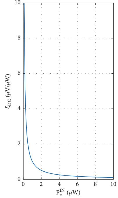
FIGURE 5: Dependence of the thermal contribution to microwave sensitivity of the spin-torque diode on the microwave input power at the a.c. current frequency of 10 GHz.
